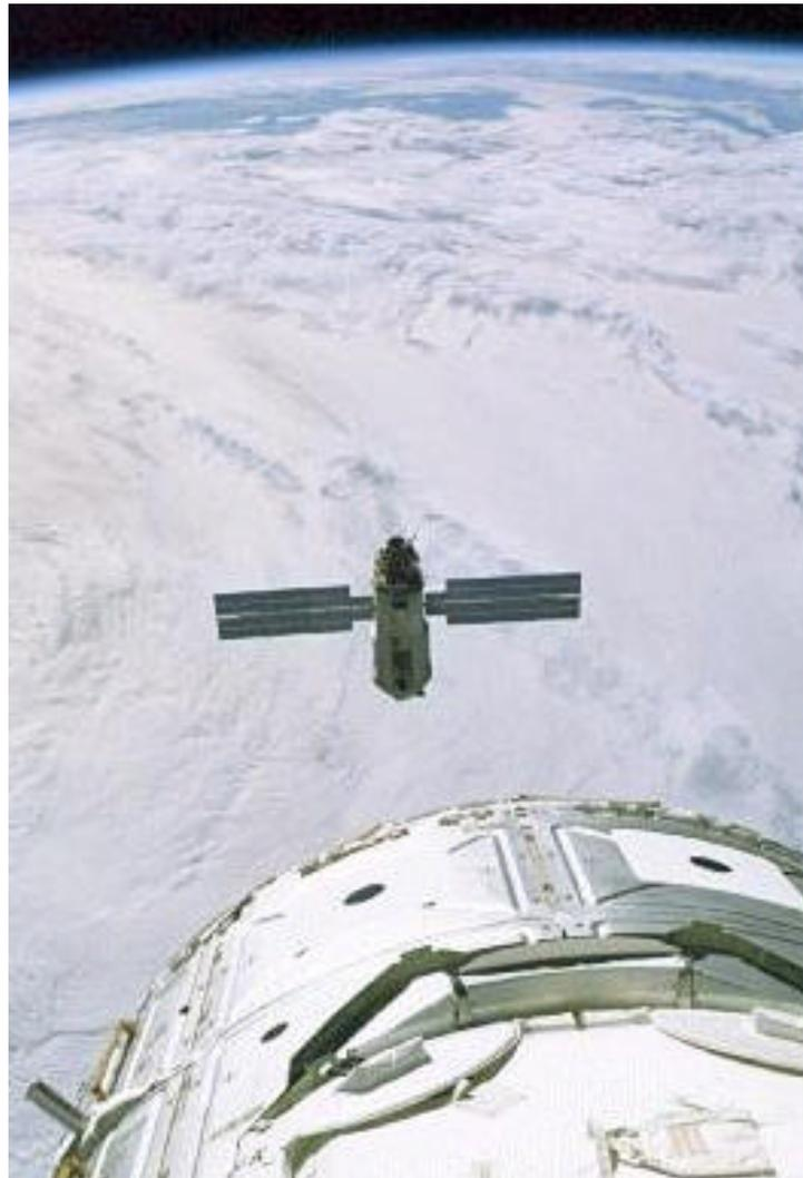
*The Zarya control module seen from the Shuttle Endeavour in December 1998 prior to attachment to the Unity connecting module. Launched from Russia, Zarya provides early propulsion and power for the International Space Station.*
