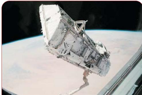
The first Integrated Truss Structure, the S0 Truss, was installed during STS-110. Mission Specialist Ellen Ochoa with assistance from Expedition Four Flight Engineer Dan Bursch used the station's robotic arm to remove the truss from the shuttle's payload bay, then install it atop the Destiny Laboratory.
