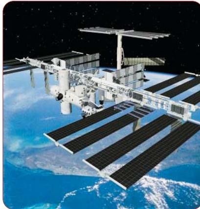
Both S1 and eventually P1 will provide structural support for the Active Thermal Control System, the Mobile Transporter, a CETA cart and antennas. The S1 has an S-band system; the P1 a UHF system. Both trusses also have mounts for cameras and lights.
