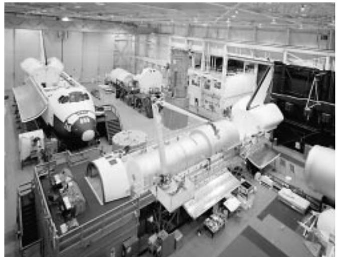
**High angle view of Building 9 Training Facilities including the Space Shuttle Full Fuselage Trainer and the Remote Manipulator System (RMS) mock-up. Also visible is a mock-up of the Hubble Space Telescope for use in training with the RMS.**
