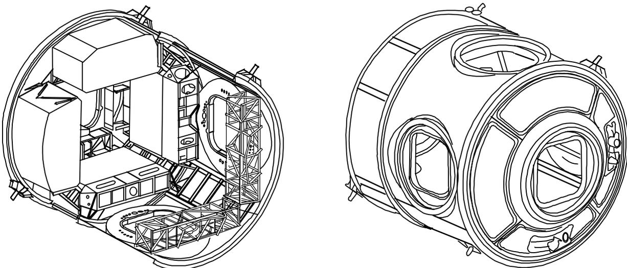
*Diagram of interior and exterior views of Unity connecting module*
